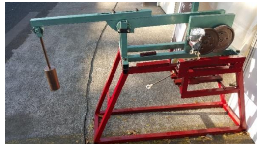
Figure 6. Construction of Two-Stage Mechanical Oscillator with Gear
