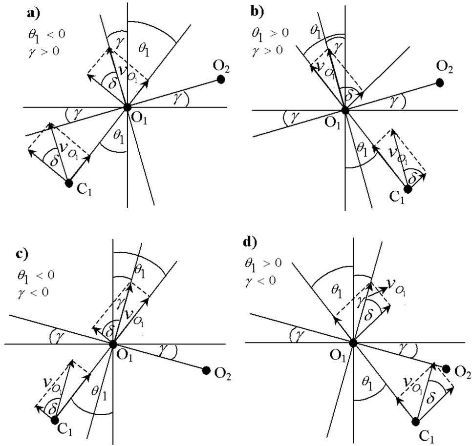
Figure 4. Angle  $\delta$  at the moment of impact
