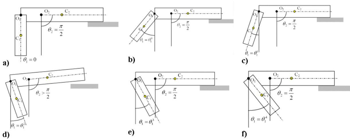
Figure 1. Characteristic positions of the double pendulum with pad during one half oscillation
