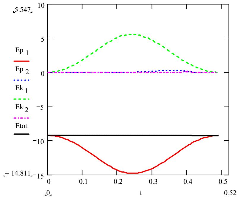
Figure 7. Potential, kinetic and total energy
