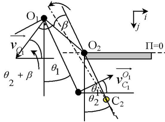
Figure 3. Characteristic points of the double pendulum with velocity vectors.
