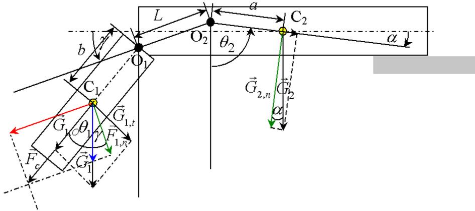
Figure 2. Forces at the moment when big pendulum is lifted of the pad
