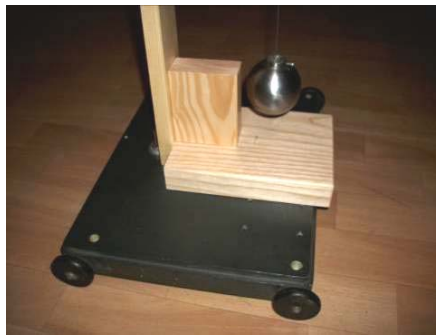
Figure 11. Elastic pendulum on a cart D = 43.2 mm (minimum amplitude)
