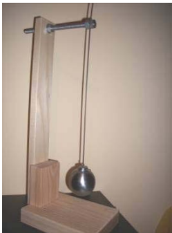
Figure 7. Elastic pendulum D = 85 mm (mean amplitude)
