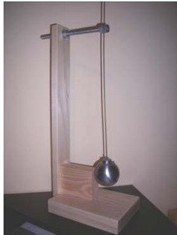
Figure 5. Elastic pendulum D = 32.2 mm (blocked pendulum)
