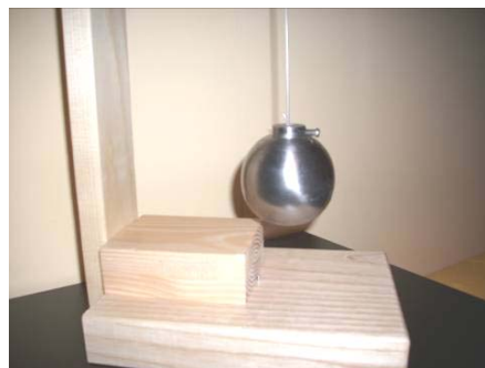
Figure 8. Elastic pendulum D = 121 mm (maximum amplitude)
