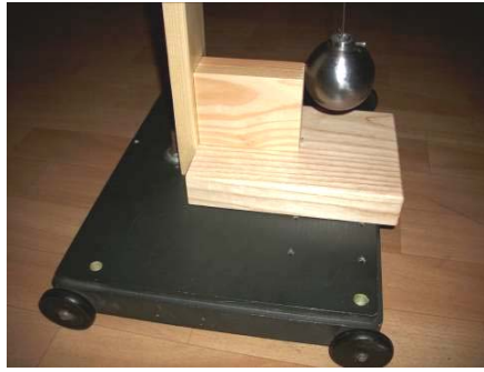
Figure 10. Elastic pendulum on a cart D = 32.2 mm (blocked pendulum)
