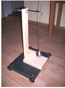
Figure 10. Elastic pendulum on a cart D = 32.2 mm (blocked pendulum)
