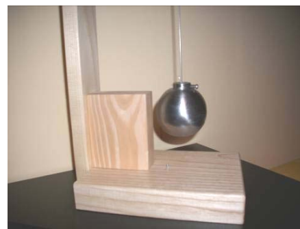
Figure 6. Elastic pendulum D = 43.2 mm (minimum amplitude)
