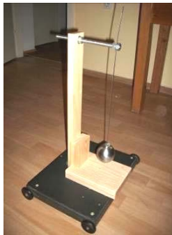
Figure 12. Elastic pendulum on a cart D = 85 mm (mean amplitude)
