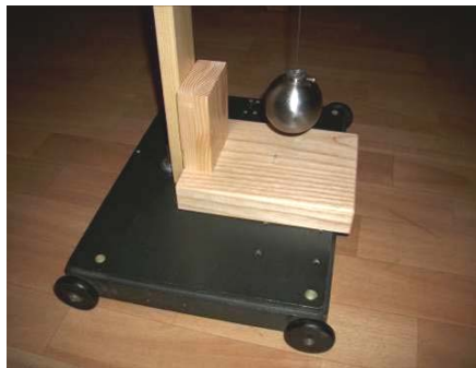
Figure 12. Elastic pendulum on a cart D = 85 mm (mean amplitude)
