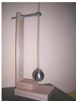
Figure 8. Elastic pendulum D = 121 mm (maximum amplitude)
