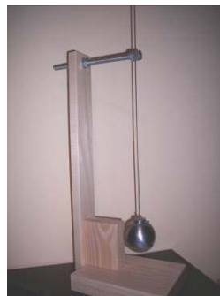
Figure 6. Elastic pendulum D = 43.2 mm (minimum amplitude)
