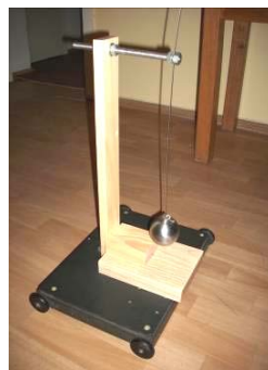
Figure 13. Elastic pendulum on a cart D = 121 mm (maximum amplitude)
