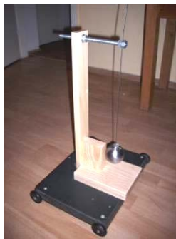
Figure 11. Elastic pendulum on a cart D = 43.2 mm (minimum amplitude)
