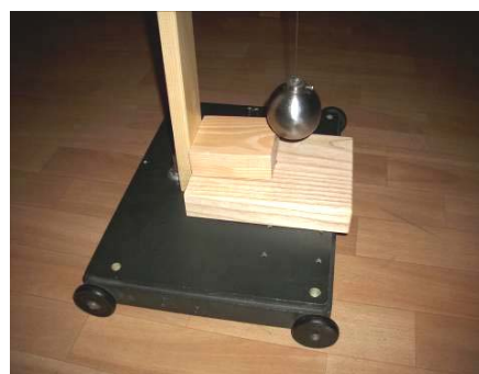
Figure 13. Elastic pendulum on a cart D = 121 mm (maximum amplitude)
