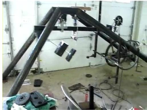
*Two Stage mechanical oscillator w 2 flywheels
