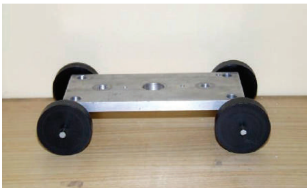
Figure 3. Experiments with small carts were performed, and due inertia they kept moving 6 - 9 seconds.
