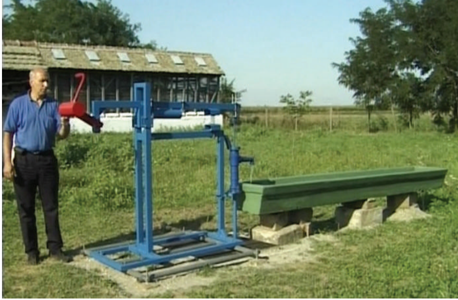
Water pump with a pendulum M. Zupkov's replica Video link: http://www.youtube.com/watch?v=hNpgl7o_1QI
