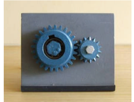
Figure 9. Transmission and reduction gears: rotation lasted 1 - 2.5 sec.
