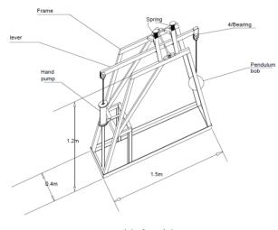
Figure 1: Model of pendulum pump.
