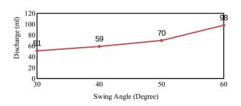
Figure 3: Discharge of water from pendulum pump vs. swing angle of pendulum.
