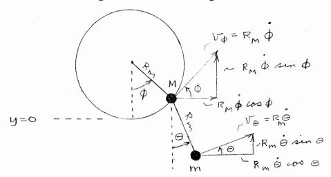
Following the procedures of (a) and (b) above, one again obtains the equations of motion, forms the expression for the energy E = T + V, and by substitution of the equations of motion into the expression for dE/dt finds here also that dE/dt = 0. Therefore, this device, as the others analyzed above, does not result in the conversion of gravitational energy into increasing device motion which could then be used to perform work.
