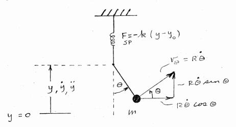
Following the procedure of (a) above, one again obtains the equations of motion, forms the expression for the energy E = T + V, and by substitution of the equations of motion into the expression for dE/dt finds that for this case also, dE/dt = 0. Once again we arrive at the result that the configuration as diagrammed above does *not* result in the conversion of gravitational energy into increasing device motion which could then in principle be used to perform work.
