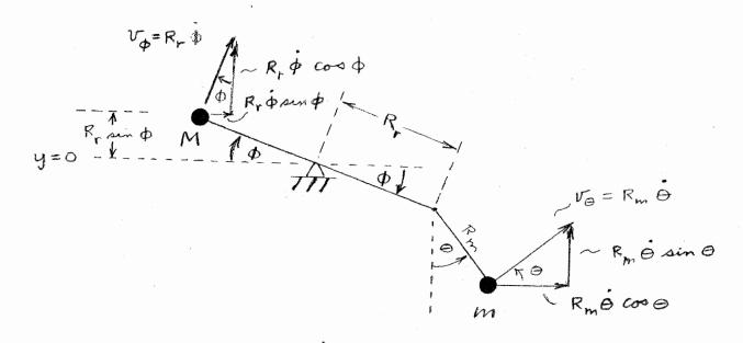
As in the previous cases, analysis by the Lagrangian technique leads to the conclusion dE/dt = 0, and therefore demonstrates that this device also does not result in conversion of gravitational energy into device motion that could result in useful work.
