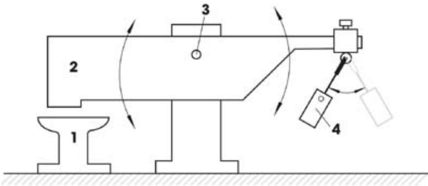
**Figure 1.** Mechanical hammer with a pendulum. 1 - anvil; 2 - massive lever; 3 - level axle; 4 - physical pendulum
