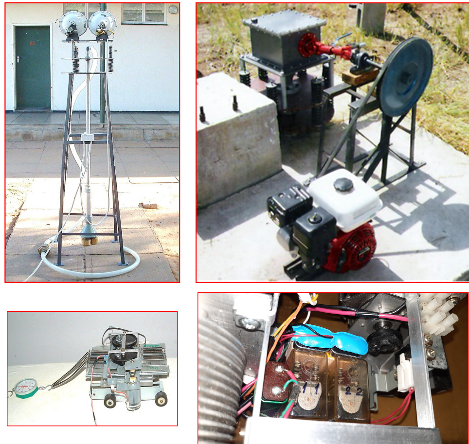
Figure 10. Devices based on professor Loukanov's activity (inertial pumps and inertial driven vehicles) (from [123–126]).
